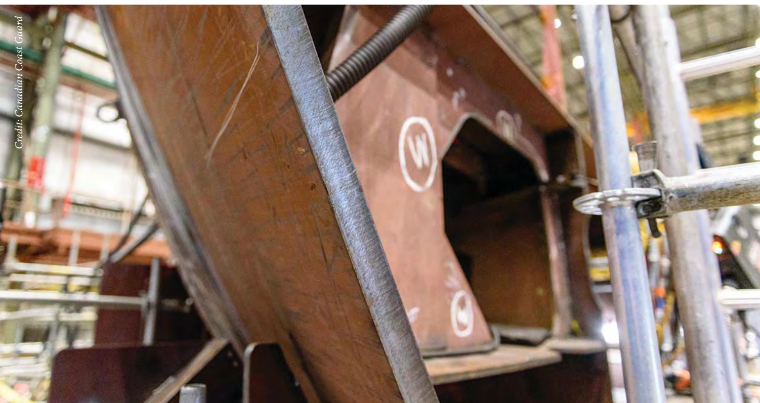
A close-up of the prototype block built by Seaspan in early 2024 using the 60 mm-thick steel that will be on the polar icebreaker. The official first steel-cutting for the ship was in April 2025.
